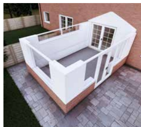
New frames and hup! walls on cill.
