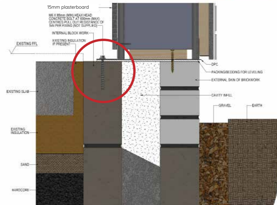
300mm Cavity Wall Base Detail (extended)
